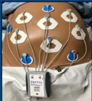
Figure 2: Schematic diagram of open-area hexagonal uEMG sensors and ECG pad placement on the gravid abdomen.
