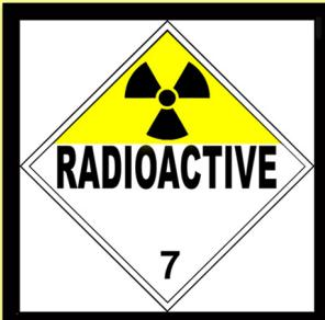
HRCQ is a high activity shipment transported in a Type B package. The package will always have a Yellow-III label regardless of radiation level. HRCQ shipments by highway will require the standard placard on a white square background with a black border as shown at left.
