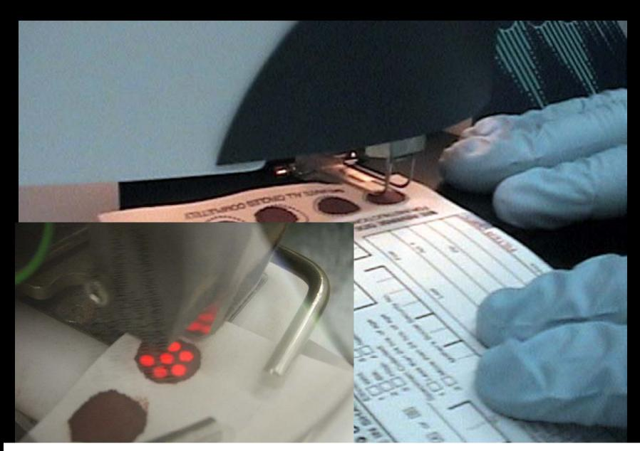
**SAMPLES ARE PUNCHED INTO 96-WELL PLATES**
