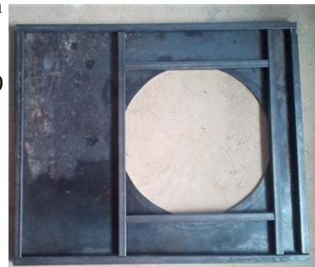
Bottom view of redesigned plancha ready for welding
